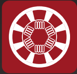
Sprung Centre Cushioned Cerametallic
